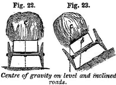
or it will immediately be thrown over by its own weight. A heavily and evenly loaded wagon on a level road will be perfectly safe, because the line of direction falls equally between the wheels, as shown in fig. 22, by the
