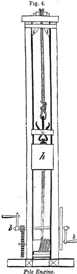
wheel-work, worked by the handles or cranks, *b b*, until the arms of the tongs which hold the ram are compressed in the cheeks, *i i*, when it suddenly falls with prodigious force on the pile or post to be driven. In this way long posts of great size are forced into the mud of swamps and
