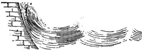
liable to injury by being built nearly perpendicular, and the waves break suddenly, and with full force, like the
