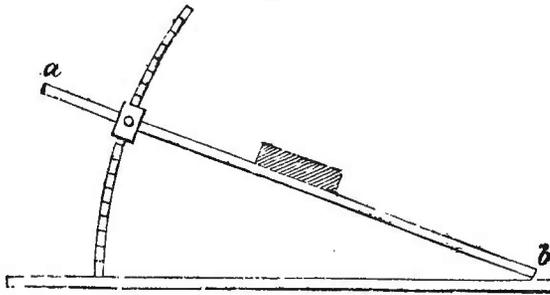
properties of the inclined plane, heretofore explained, that it requires a force equal to one-half the weight of the wooden block to slide it over a smooth wooden surface. Some kinds of wood have more friction than others, but this is about the average.\*
