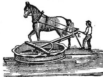
pressure is completed, the driver touches the upright rod, and detaches the wheel or drum, by which the rope is drawn backwards, without stopping the horses, which continue to walk around the circle.
