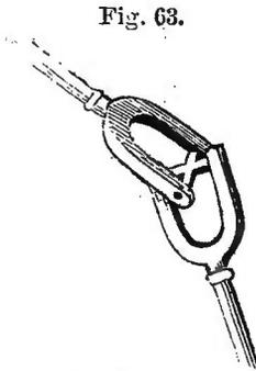
municated by means of the *universal joint*, as shown in fig. 63. This is commonly used in the thrashing-machine, where there is a slight change in the direction of motion between the horse-power and the thrasher.
