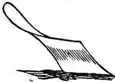
It will be readily understood, however, that more force will be needed for drawing a short or blunt plow, like Fig. 131, than one in the form of a longer wedge, as in fig. 132, the latter, like a sharp boat in water, moving more easily. Care
