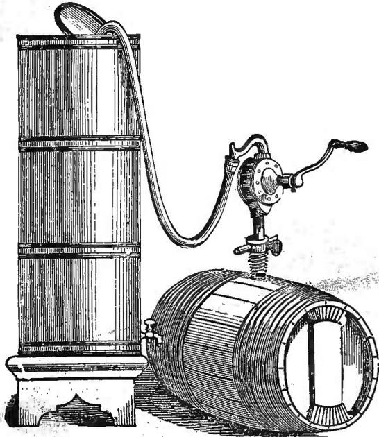
*Rotary Pump, for Barrels, etc.*
