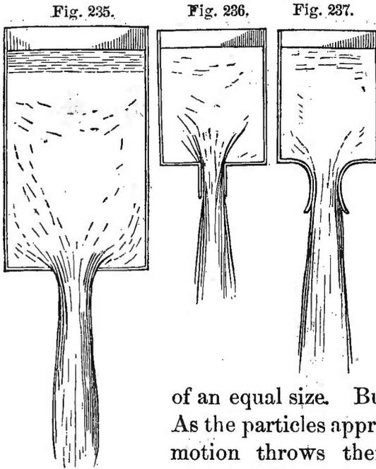
If, for example, a vessel or cistern have a thin bottom of tin, with a smooth, circular hole, we might naturally suppose that the discharge would be as easy as it could be made, and that water would pass as rapidly through it as through any orifice
