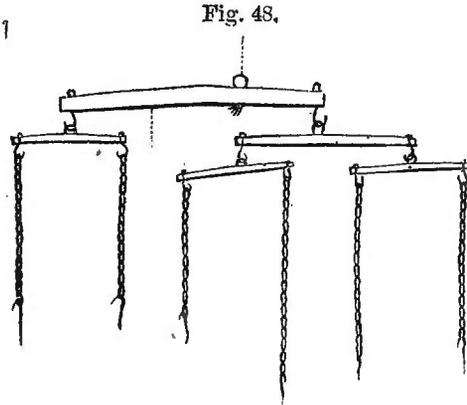
worked abreast, the two horses placed together should have only half the length of arm of the main whiffle-tree as the single horse, fig. 48.
