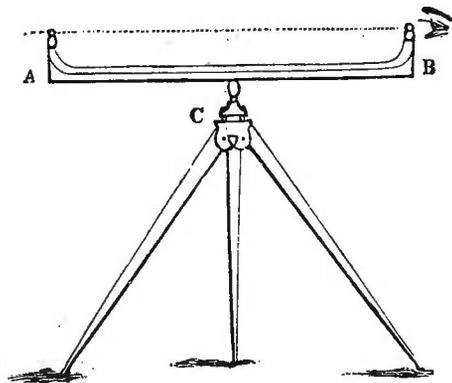
When the bar is made perfectly level, as shown by the air-bubble, by sighting through at the two wires, the levelness or descent of the land may be determined.
