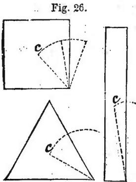
Of all forms, a pyramid stands the most firmly on its base. The centre of gravity, *c* (fig. 26), being so near the broad bottom, it must be elevated in a very steep curve to throw the line of direction beyond the base. For this reason, a stone wall, or the dam for a stream, will stand better when broad at bottom and tapering to a narrow top than if of equal thickness throughout.
