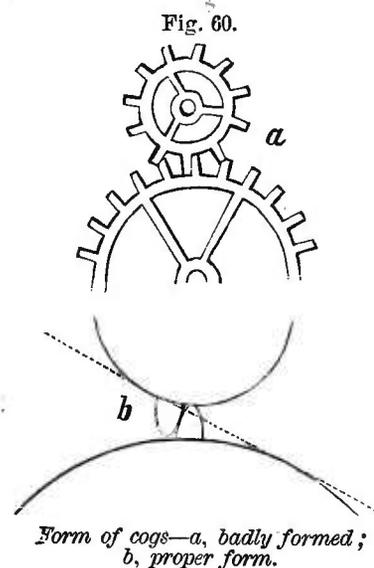
formed separately and inserted into the wheel, as with wooden wheels. *Pinions* are the small wheels, or, more properly, teeth set on axles.
