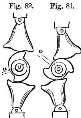
are at first near together, but are crowded asunder as the lever is pressed downward. This cheese-press is made of cast-iron, and has great power; to try it, weights were increased upon the lever, until the iron frame broke with a force equal to sixteen tons.
