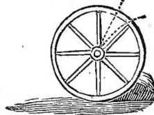
run with more ease on a rough road than a smaller one; the larger one mounting any stone or obstruction without lifting the load so much out of a level or direct line, as shown by the dotted lines in the annexed figures, (figs. 29
