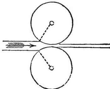
*Principle of the knee-joint in the rolling-mill.*
