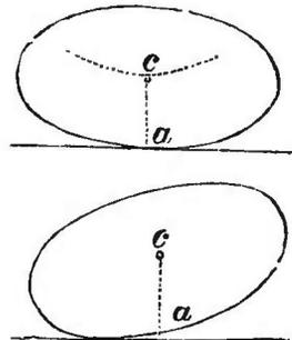
If it be placed upon end, as in fig. 38, then any motion toward either side brings the centre of gravity nearer the touching-point, that is, causes it to descend, and the body consequently falls over on its side. This may be easily illustrated with an egg, which will lie at rest upon its side, but falls when set on either end.
