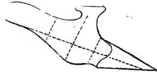
But there are two objections to this form in practice. The first is that the sod is laid over smoothly and unbroken, and without being at all pulverized. On heavy and hard soils this is a serious fault. The other objection is that the sod is elevated as rapidly at the first movement, when its weight is considerable, as just before falling, when its pressure on the mould-board is slight. These difficulties are in part removed by giving the mould-board a
