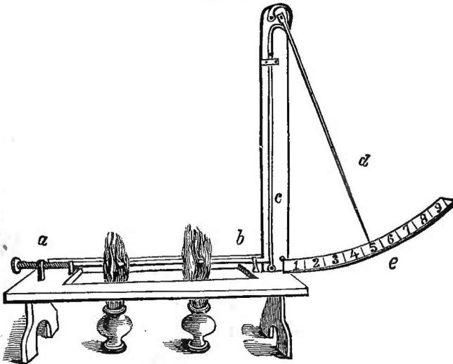
into the hole. The expansion may be more visibly shown and accurately measured by means of an instrument called the *Pyrometer* (fig. 288). The rod *a b*, secured to its
