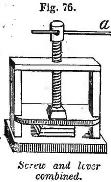
screw, here is another increase of twenty times in force. Multiplying 20 by 20 gives 400, the whole amount gained by this combination, and by which a man applying one hundred pounds in force could exert a pressure equal to twenty tons. About one-third or one-fourth of this should, however, be deducted for friction.
