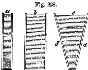
for instance, the vessel *a* (fig. 228), be one inch in diameter, and the vessel *b* be three inches in diameter, the water being equally high in both, the pressure on the whole bottom of *b* will be nine times as great as on
