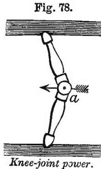
the levers is fixed to a solid beam, and the other connected with a movable block. When the joint *a* is forced in the direction indicated by the arrow, it produces a powerful pressure upon the movable block, which in-
