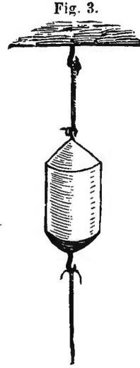
If the jerk be very sudden, the lower string will break, even it be considerably stronger than the upper, the *inertia* of the weight requiring a great force to overcome it suddenly. The threads used in this experiment may be easily had of any desired strength by taking the finest sewing cotton, and doubling to any desired extent.
