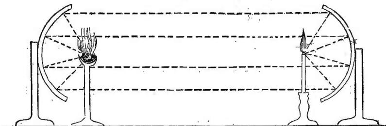
the dotted lines (fig. 295), and, setting fire to the phosphorus, will light the candle.
