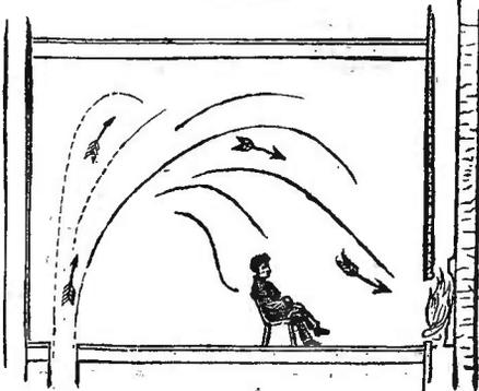
Hence the importance of the admission of currents of fresh air into all occupied rooms, by means of ventilation.
