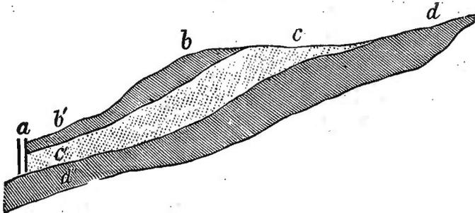
rain falls upon the surface, as at *c d*, it sinks down in the more porous parts between these layers, to *c*. If the layers happen to be broken in any place below, the water finds its way up through the crevices by the pressure of the head above, and forms springs. If there are no openings through the rocks, deep borings are sometimes made
