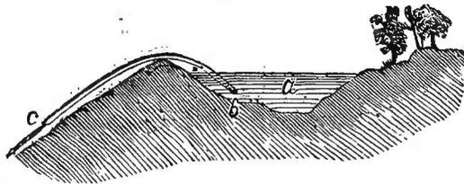
instance, let *a* (fig. 267) represent a body of water which it is desirable to drain off; by placing the lead tube, *b c*, so that the arm, *c*, may be lowest, and applying a pump at this arm to withdraw the air and fill the syphon with water, it will commence running, and continue until the
