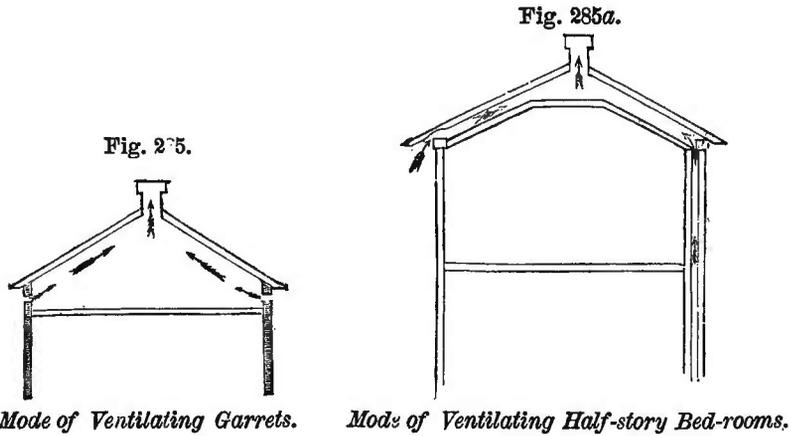
and admitting air at windows or openings near the eaves (fig. 285), thus sweeping all the hot air out by the current produced ; or the oppressive heat of half-story bed-rooms may be similarly avoided, by creating a current of air between the roof and the plastering (fig. 285a). Two modes may be adopted, as represented on each side of the figure.
