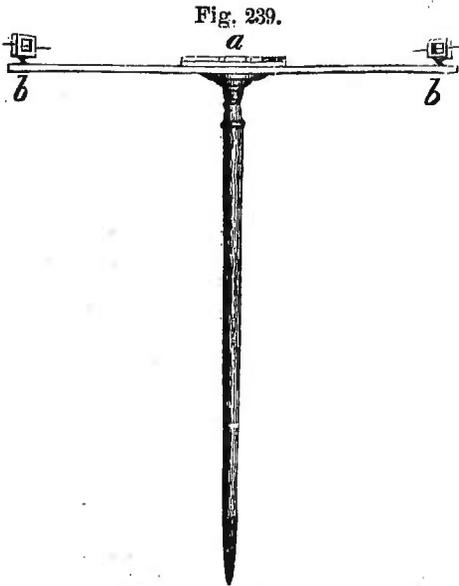
Procure a mason's or carpenter's spirit-level, (*a*, fig. 239) fasten it to the upper side of a straight bar of wood, and on the ends of this bar secure small, upright pieces of tin plate, *b, b*, having openings cut in the centre. Horizontally across these openings, draw very fine wire, which shall be exactly at equal heights above
