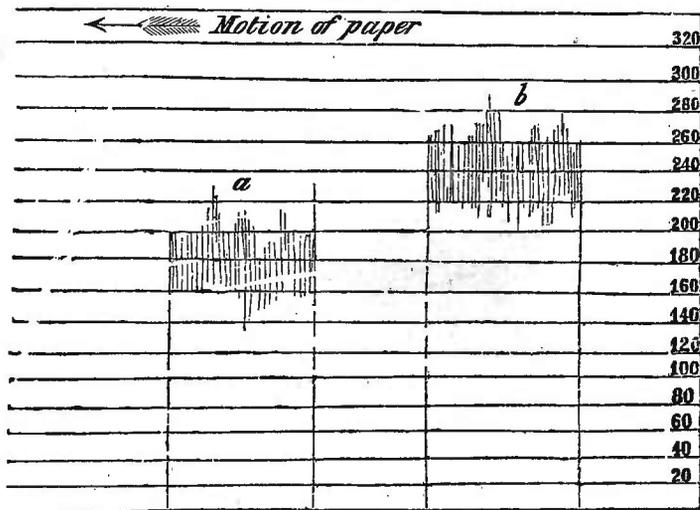
The markings of the Self-recording Dynamometer.
