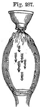
just above the bulb, may be set on fire, and will continue to burn for some time before any effect can be seen upon the thermometer. The upper surface of a vessel of water has been made to boil a long time with a piece of unmelted ice at the bottom. Liquids are found, however, to possess a conducting power in a very slight degree.
