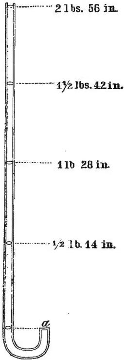
inches; two pounds, fifty-six inches; ten pounds, twenty-three feet; twenty pounds, forty-six feet, and so on. Now, as the side pressure is the same as the pressure downward for the same head of water, the same column will, of course, exert an equal pressure on a square inch of the *side* of the tube. Or, if the tube be bent, as shown in the annexed figure (fig. 226), the pressure upward on the end of the tube, at *a*, will be the same for the various heights.
