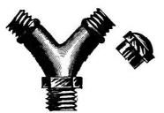
FIG. 266.—Y-Fixture for Vermorel Nozzles. FIG. 267.-Y-Attachment for using
