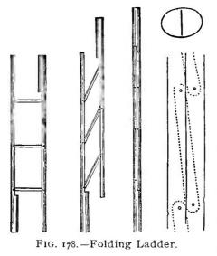
carried in one hand. It is made of strong, light wood, and its construction may be readily un derstood by the annexed figure (Fig. 178), representing the ladder as open, as half-closed, and as closely shut. An enlarged longitudinal section shows the manner in which the rounds lie in the grooves or concave beds in the sides or styles; above which is a cross-section exhibiting the semi-oval form of the styles. The ends of the rounds turn on iron pins, slight-
