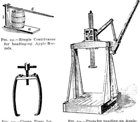
FIG. 193.—Cheap Press for heading-up Apple-Barrels.
