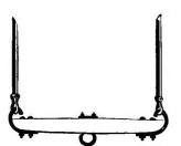
It is made as short as the free action of the animals' legs will allow (about sixteen inches for a single whiffletree). An iron strap is riveted so as to bend round the end of the wood, turning in and forming a hook inside.
